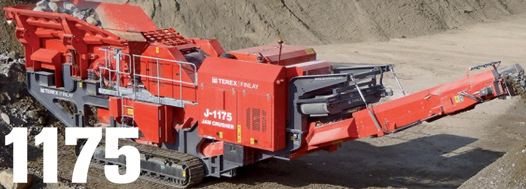
The Terex Finlay J-1175 is a high performance tracked mobile jaw crusher. Incorporating the Terex Jaques JW42 jaw crusher and a heavy duty VGF feeder the Finlay J-1175 gives optimum production in a range of applications.
