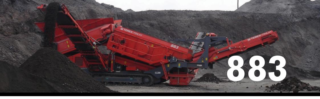
The high performance Terex Finlay 883 is designed to work after a primary crusher or on it's own as a frontline tracked mobile screening machine. Applications include quarrying, mining construction and demolition debris, topsoil, recycling, sand, gravel, coal and aggregates. The plant has the capacity to process at a rate of up to 500 tonnes per hour and can be fed either by a tracked mobile crusher or an excavator.
